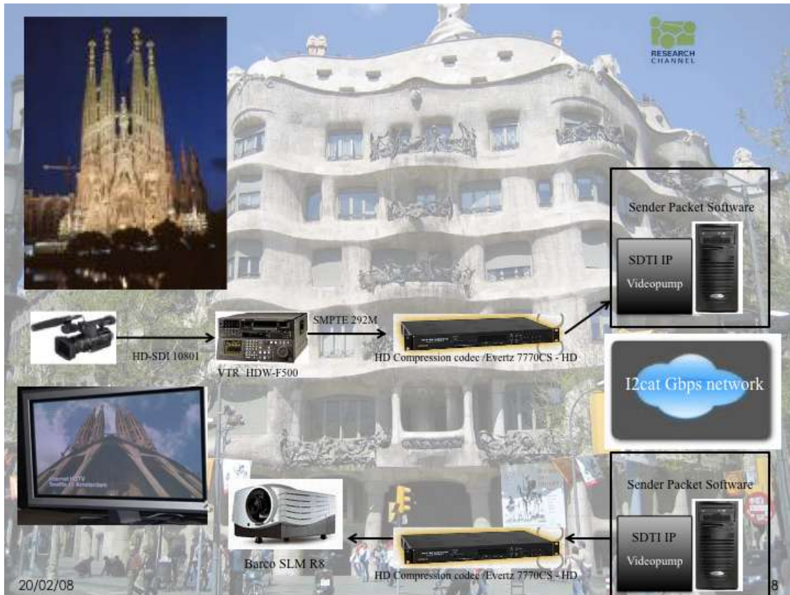
HD Gaudi, 2002: First compressed HD live transmission between Europa-USA over Internet at 270 mbps by i2CAT-Research Channel
